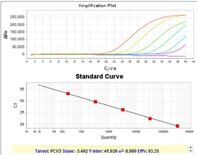
Fig. 1 The amplification plot of PCV3 capsid plasmid with the concentration of  $10^6$ ,  $10^5$ ,  $10^4$ ,  $10^3$ ,  $10^2$  and  $10^1$  copies/ $\mu$ L. The standard curve plotted against the Ct values in amplification plot (linear range:  $10^2 - 10^6$  copies/ $\mu$ L,  $R^2 = 0.999$ )
