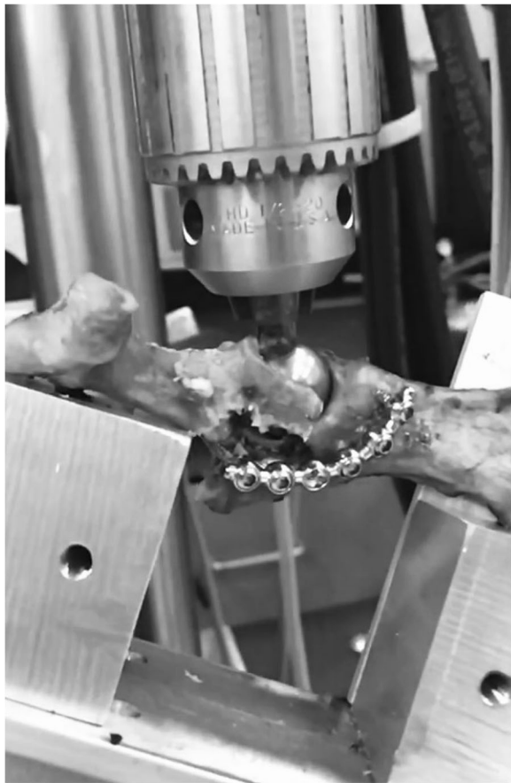
Fig. 3 String-of-Pearls™ construct failure via caudal screw cut-out
