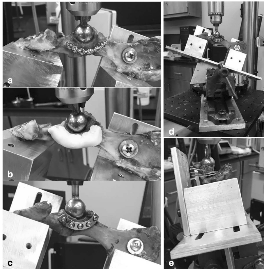
Fig. 4 a String-of-Pearls™ plate contouring, application, and mounting. b Screw/Wire/Methylmethacrylate fixation demonstrating application and mounting. c Veterinary Acetabular Plate application and mounting. d Demonstration of the testing apparatus to replicate 110° hip flexion. e Demonstration of the testing apparatus to replicate 105° hip abduction
